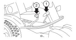
3 Select the required cutting height (1-7) with the cutting height lever.
